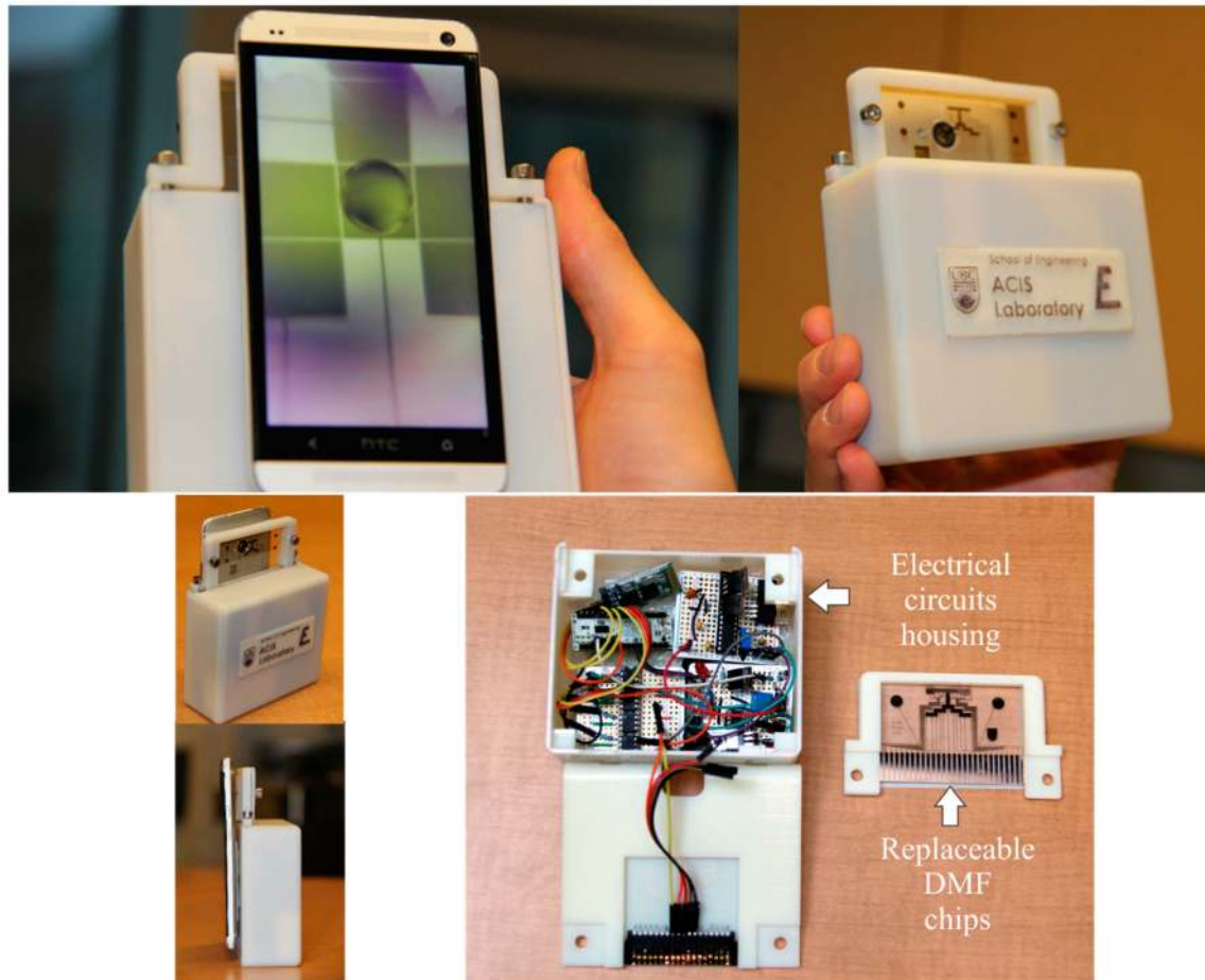
Figure 8. The final prototyped portable DMF modular platform.
