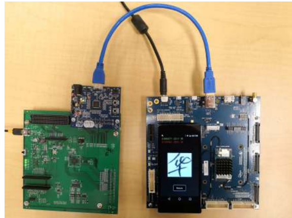
Figure 5. OCR on CNN-DSA accelerator connected to mobile platform.
