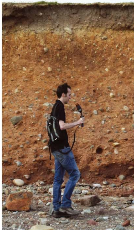
Figure 1. The Zeb1 hand-held mobile laser scanner (HMLS) in use at the coastal cliff site Sunderland Point, UK.
