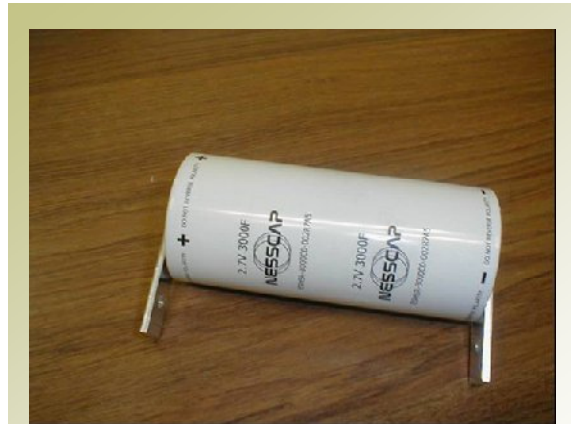
Figure 2 The NessCap 3000F capacitor
