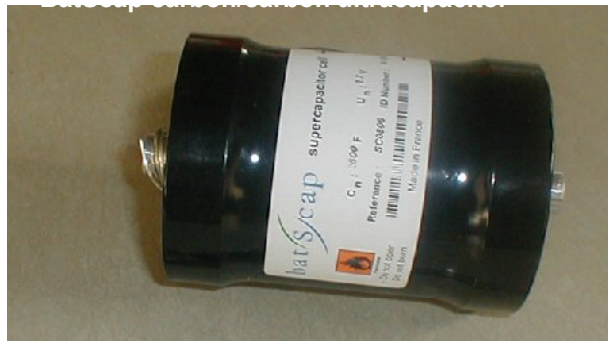
Figure 3 The Batscap 2700F capacitor
