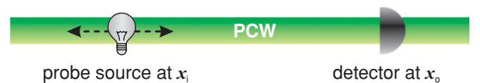
FIG. 4. (Color online) Model schematic of the experimental situation. The pointlike probe laser with linear polarization e_i and a detector are placed next to the input and output facet of the waveguide at positions x = x_i and x_o .
