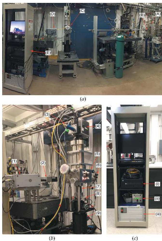
Figure 2 Photographs of the experimental setup. (a) Overview of the 32-ID-B beamline at the APS. (A) Slow shutter, (B) fast shutter, (C) laser AM experimental setup, (D) high-speed X-ray imaging setup, and (E) laser system control computer and laser source rack. (b) Detailed view of the setup. (1) High-speed camera, (2) scintillator–mirror–objective lens assembly box, (3) laser feeding fiber and collimator, (4) laser scanner, (5) experimental chamber, (6) connection for the vacuum pump, (7) vacuum-compatible bellows, (8) three-axis translational stages for sample manipulation, and (9) two-axis stage for laser–X-ray alignment. (c) A detailed view of the control rack. (i) Scanner control computer, (ii) power sources and connection boxes for the scanner, and (iii) laser source.
