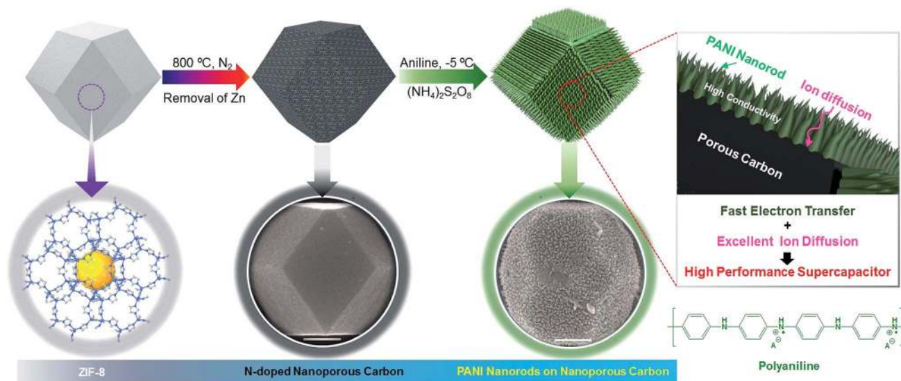
Scheme 1 Schematic illustration of the synthetic process for the attainment of nanoporous carbon–PANI core–shell nanocomposite materials, starting from the rhombic dodecahedron ZIF-8. For the preparation of nanoporous carbon, ZIF-8 was carbonized and Zn was removed by washing with HF. The SEM images of the bare carbon and carbon–PANI nanocomposite are as shown. The scale bars are 500 nm in length. The PANI nanorods were grown on nanoporous carbon and the lengths of the nanorods were controlled by the polymerization time.
