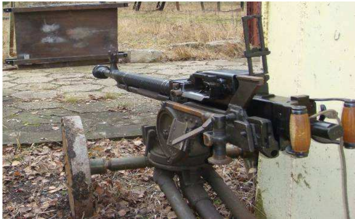
Fig. 3. Stand for tests of protection ability of maraging steel plates placed on an RHA witness plate
