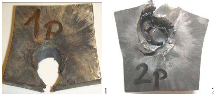
Fig. 6. Frontal view of maraging plates (shot no. 1 and 2) following firing with 12,7 mm type B-32 AP projectile
