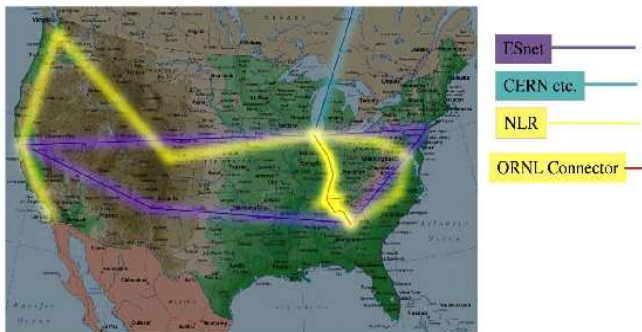
Fig. 1. UltraScience Net backbone consists of dual 10 Gbps lambdas from Atlanta to Chicago to Seattle to Sunnyvale.
