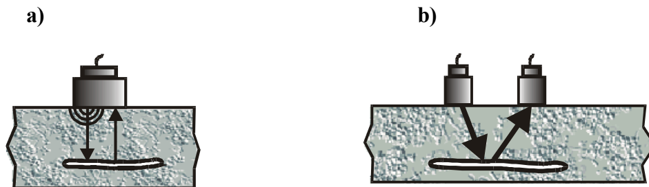
Figure 3. Testing the concrete by ultrasonic echo method: a) transmitting-receiving transducer, b) double transducer
