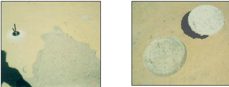
Figure 20. Example of deteriorated industrial floor and evaluation of adhesion with pull-off test
