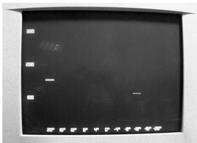
Fig. 6. Experiment-II. A good reflector is placed 150 cm away from the device with an angle of 20^\circ . A bad reflector is placed 120 cm away from the device with an angle of -12^\circ . The good reflector appears brighter and the bad reflector appears dimmer in the image. The image has 21 dB dynamic range.
