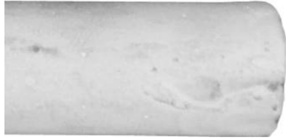
Fig. 5.5. Radiator surface with Z-Guard coating. No metallurgical bonding was observed. The bonding between the coating and radiator surface was excellent.
