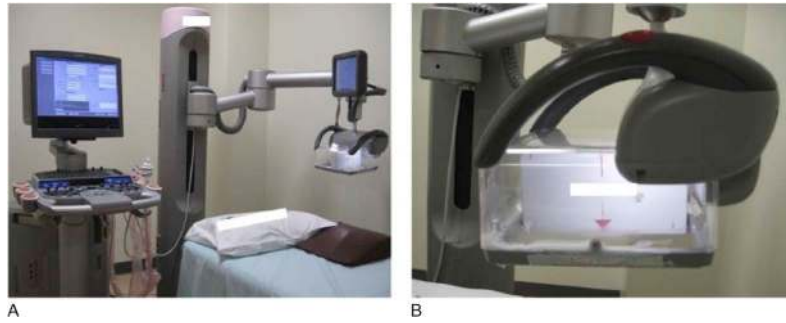
Figure 9. Automated breast volume scanner: (A) Acuson S2000 ABVS (Siemens Medical Solutions). The transducer plate (B) is positioned over the breast and an automated scan is performed in order to obtain a series of two-dimensional images. Depending on the breast size, more than three scans per breast may be required. Reprinted from (Shin, et al. 2015).
