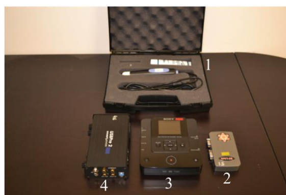
Figure 4: Ultrasound equipment (1: Ultrasound probe, 2: PC-TV converter, 3: DVD recorder, 4: SOUND DEVICES USBPre2 pre-amplifier)
