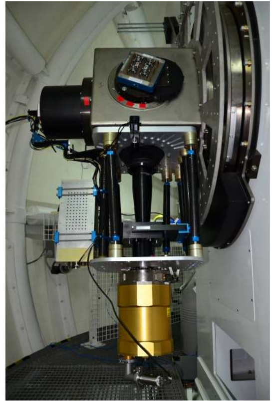
Figure 4. Left: mechanical drawing of the ULTRASPEC optomechanical chassis, highlighting some of the components shown in the photograph on the right and described in the text. Right: photograph of ULTRASPEC mounted on the Nasmyth focus of the TNT. The length and mass of ULTRASPEC, not including the Nasmyth cube, are approximately 1.0 m and 90 kg.
