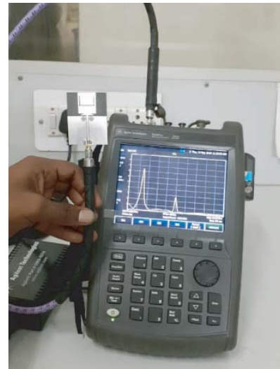
Figure 8. Antenna measurement using VNA.
