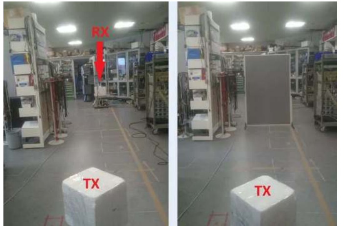
Fig. 6. Measurement scenario. Left in the figure the LOS case is shown and right in the figure the O-LOS case is shown. The biconical TX antenna, seen in the bottom of both scenarios, is encased in styrofoam as a part of its design.
