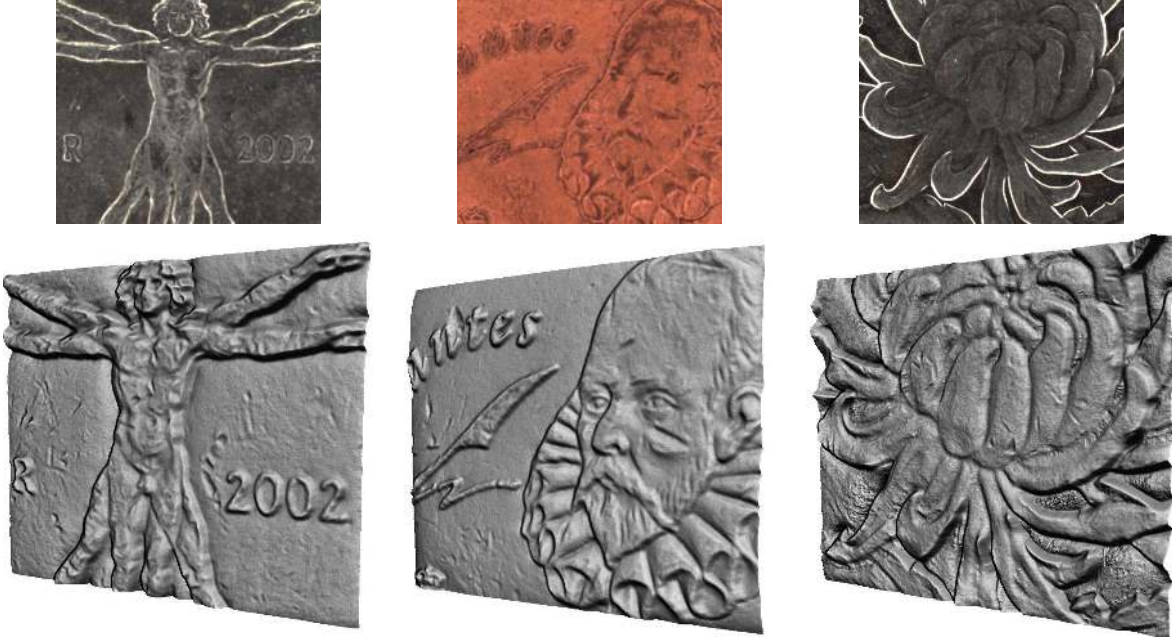
Figure 5. 3D-reconstructions of three metallic coins: an Italian euro, a Spanish 50 cents coin and a Chinese yuan. Each reconstruction domain is around 1 \text{ cm}^2 . Top: one of the m = 5 input images. Bottom: 3D-reconstruction result. Metals are successfully handled, despite the Lambertian assumption and the choice of least-squares estimation.
