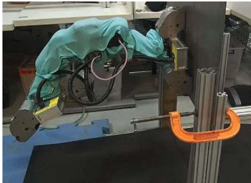
(a) Inchworm robot at the initial pose in the partition plate environment.
