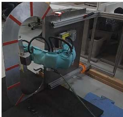
(e) Final inchworm robot pose in the manhole environment.
