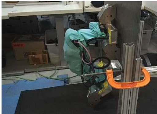
(c) Inchworm robot in a pose prior to repulsive force pushing the end-effector away from the partition plate.
