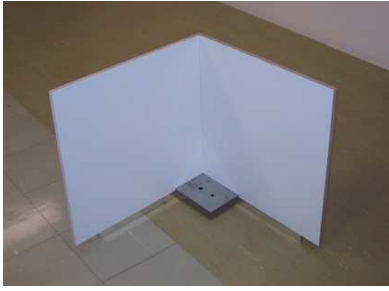
Figure 8: Laser calibration tool – “perfect” corner.
