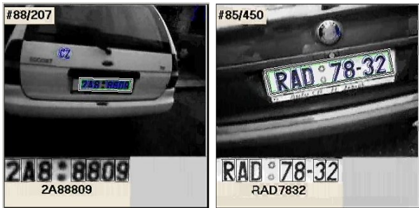
Fig. 3. Licence plate detection and recognition. Detected CSER are highlighted by blue color, the appropriate longest linear configuration is highlighted by green color. Then the detected LP is normalized and recognized by standart OCR method.
