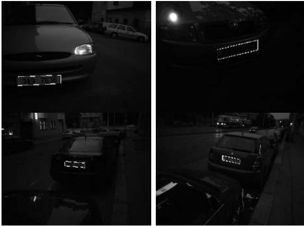
Fig. 5. (a) The classifier output for character-like region and non-character region. The Figure shows that classification of letter is robust to illumination change. The growing region is classified as character over a very large range of thresholds (40–160). (b) Licence plate detection in night shows brightness invariance of proposed method.
