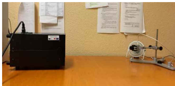
Figure 2. Disposal of the blackbody and the camera for calibration.
