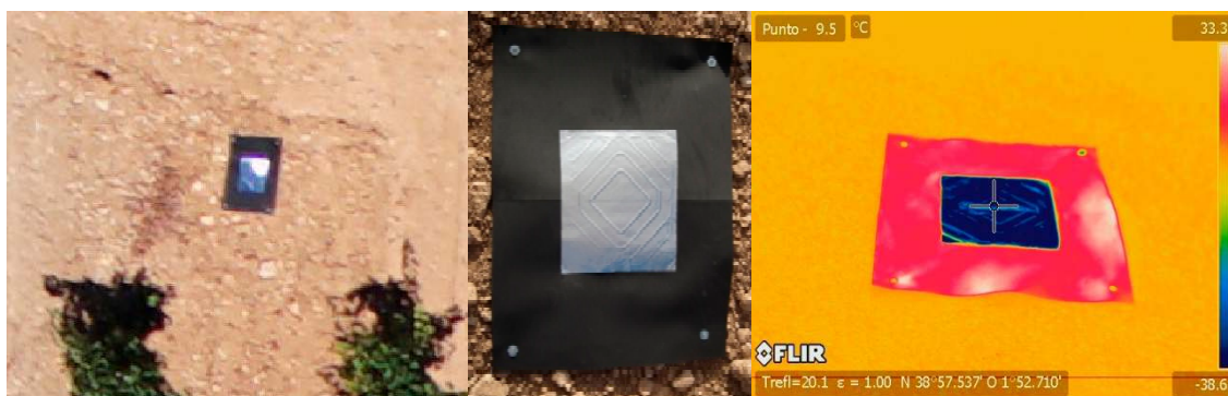
Figure 6. Type of GCPs used in thermal images.
