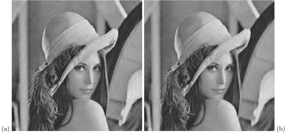
Figure 1: A result from the shift4 algorithm with and without post filtering. (a) shift4 , \sigma = 20 , 4 levels. MSE=93.17. (b) the image in (a) followed by 3 \times 3 mean filter. MSE=66.11.
