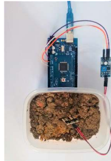
Figure 4: Prototype of the underground soil moisture sensor for data gathering.
