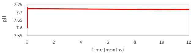
Fig. 10 The evolution of pH as a consequence of hydrogen injection within 1 year (obtained from the final kinetic model; A_{sp} specific contact area ( \text{cm}^2/\text{kg} water):1; rate constant ( \text{mol}/(\text{cm}^2\text{s}) ): 1\text{e-}7 ; injected \text{H}_2 fugacity: 7.5 bar)
