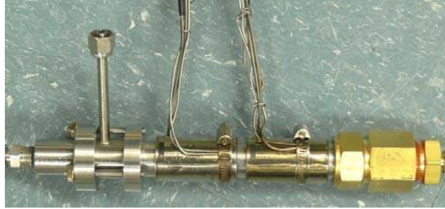
Figure 23. Photograph of liquid fuel vaporizer, with externally clamped electrical heaters. The side port tubing is for nitrogen purging of the system.
