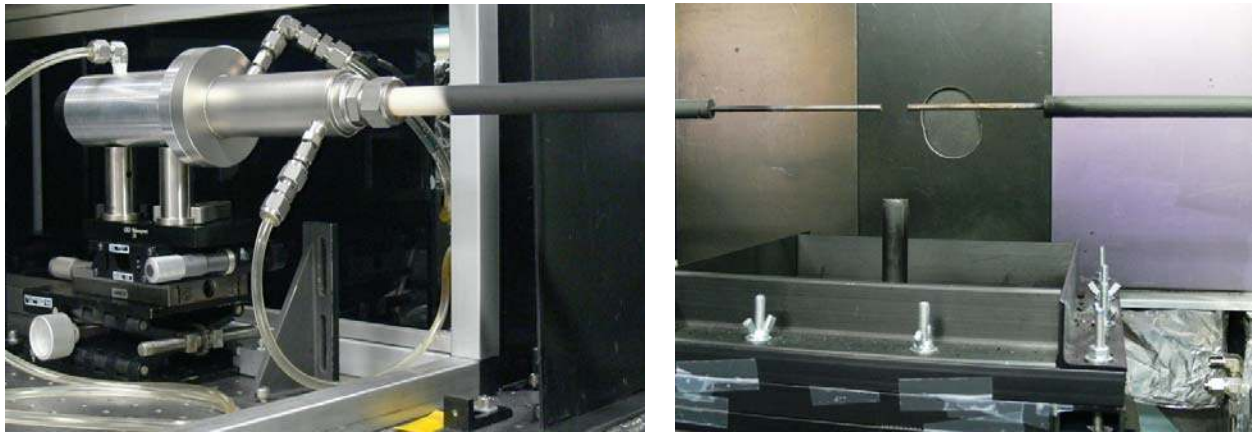
Figure 44. Optical probe for performing 3-line measurements of soot temperature/concentration statistics in the turbulent jet flame. Aluminum optical housing (left) is water-cooled and provides N_2 purge gas. Refractory probe ends (right) are uncooled.
