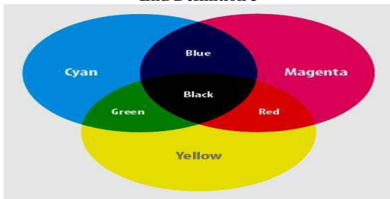
Figure 8: CMY (K) subtractive color model representation [5].
