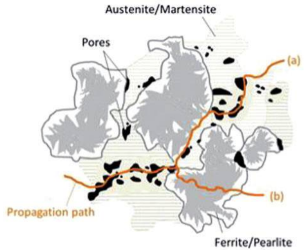
15 Model of crack propagation path through microstructure of DAE
