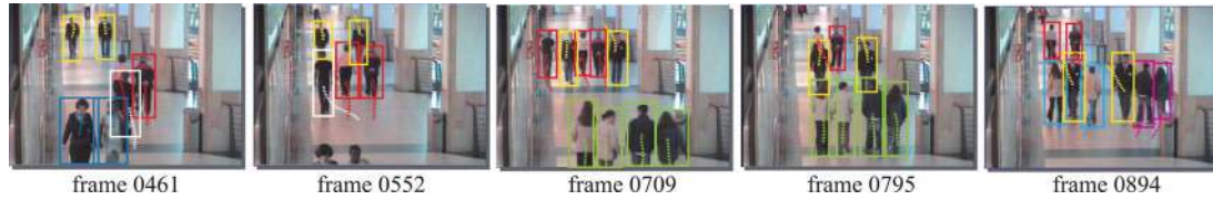
Fig. 5. Group detection results from CAVIAR dataset. The pedestrians that are walking in the same group are marked in the same color. The splitting and merging behaviors are shown in the last four frames.
