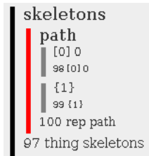
Figure 34: A skeleton with all three types of skeleton options: rep path is a constant Thread; [0] 0 points to the Thread of the first frame’s first component and {1} points to the entire second frame.
