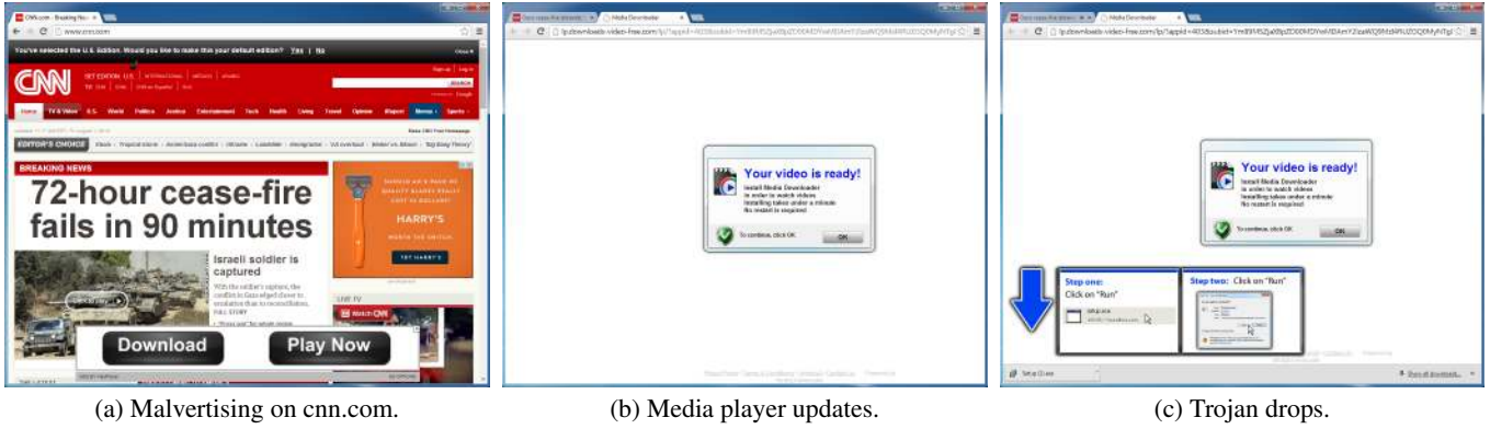
Figure 5: Extension Plus-HD 1.3 inserts a malicious ad on cnn.com, pop ups media update warning and drops a Trojan on the unwary user machine.
