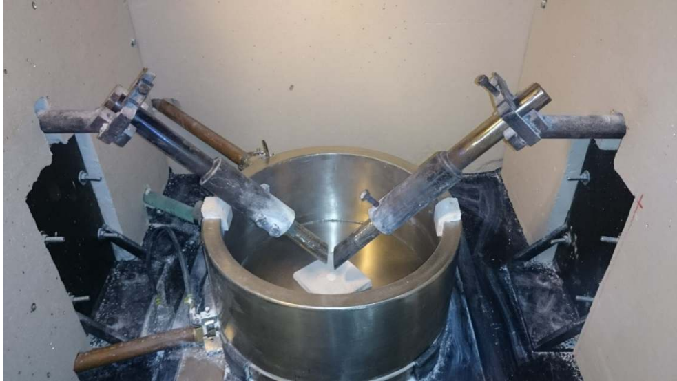
Figure 3.1: Melt furnace (344 mm interior \varnothing and 160 mm height) and molybdenum glass melting electrodes (52 mm outer \varnothing and 200 mm long).
