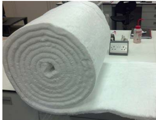
Figure 2.3: Superwool XT® needed blanket (BG-15-P19-7702) with 128 \text{ kg/m}^3 density.
