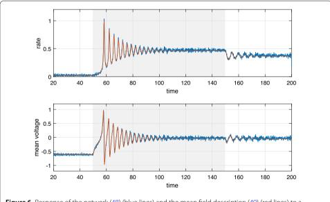
**Figure 6** Response of the network (48) (blue lines) and the mean field description (49) (red lines) to a transient input turned on at t = 50 and off at t = 150 (shaded background). A network of 1000 neurons was used and the data from the network was smoothed by convolution with a Gaussian of standard deviation 0.05 time units before plotting
