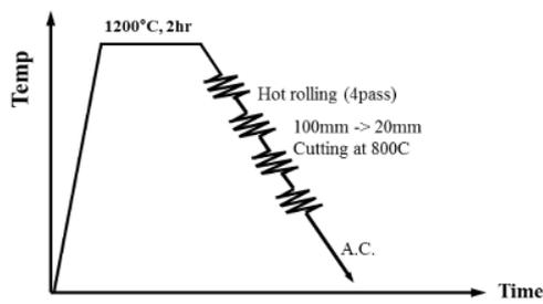
Fig. 1. Cooling curve
