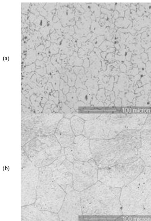
Fig. 3. Optical micrographs (a) 800°C, (b) 1350°C
