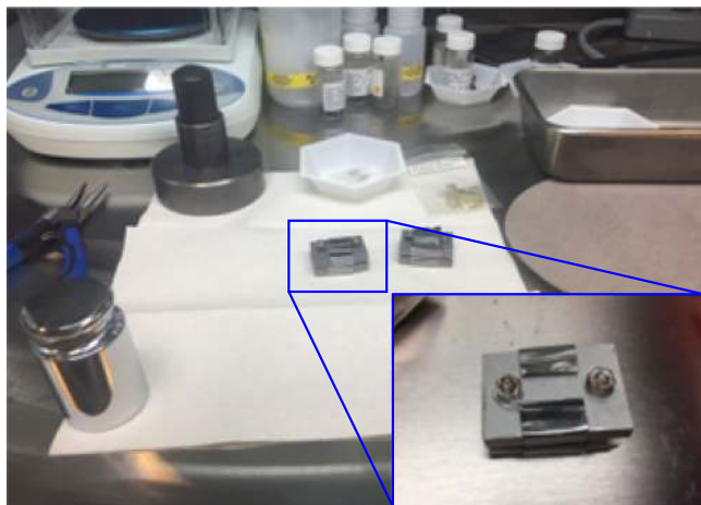
Fig. 4 Diffusion couple setup. Diffusion couple fixed in a molybdenum-jig inside a glovebox.
