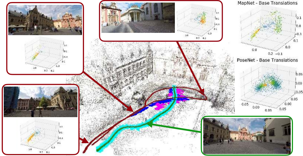
Figure 1. Visualization of the base translations \{c_j\} learned by PoseNet [29, 30] and MapNet [11]. Each point corresponds to one base translation. The scale of the base translations is in meters. We show the combinations of base translations for some training images for MapNet. The weight a translation received in Eq. 3 for a single image, respectively all images (on the right of the figure), is indicated by colors and point sizes, with warm colors and large points for translations with a large coefficient. The training and test trajectory are shown in red and green. The test predictions by PoseNet and MapNet and Active Search [59] are shown in blue, purple, and cyan, respectively.
