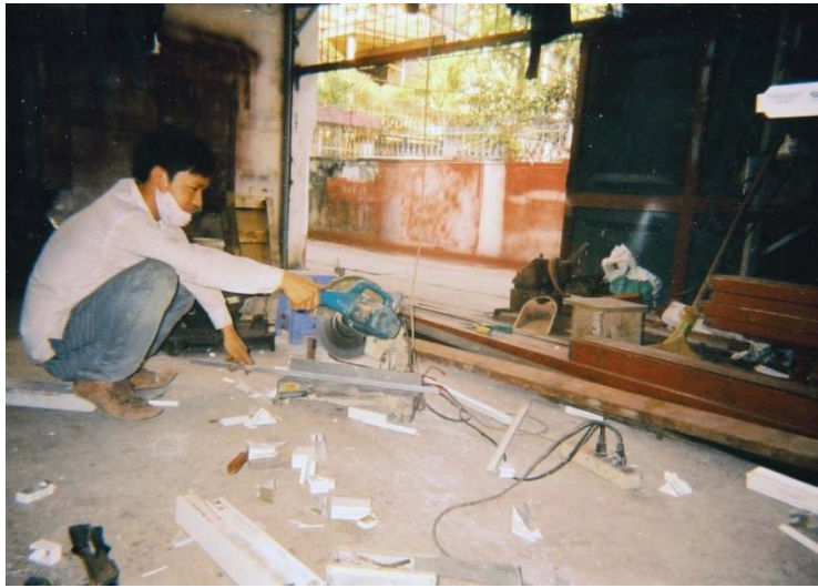
Photo 6.12. Cutting a metal bar at work (Photo by Duc, 24, male, construction worker)
