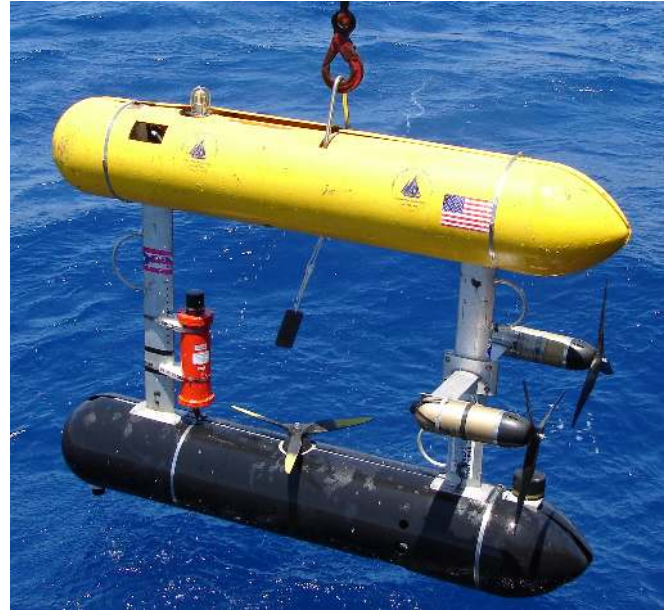
Fig. 1. The SeaBED AUV, developed at Woods Hole Oceanographic Institution, uses the Micro-Modem for telemetry and navigation. It currently can perform narrow-band LBL ranging, and acoustic telemetry synchronous ranging, which is used to correct its DVL assisted dead-reckoning. SeaBED is designed to make high resolution photo mosaics, do multi-beam bathymetry and also carries a suite of chemical and oceanographic sensors.
