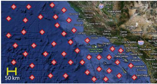
Fig. 1. Representative example of a sensor deployment on the ocean floor to monitor environmental conditions. Such sensors remain in place for many months. Retrieving data from the sensors during deployment is challenging due to limited communication underwater. A mobile AUV equipped with an acoustic modem can act as a data collection device in this scenario by traversing a path that minimizes travel time and maximizes information gathered.
