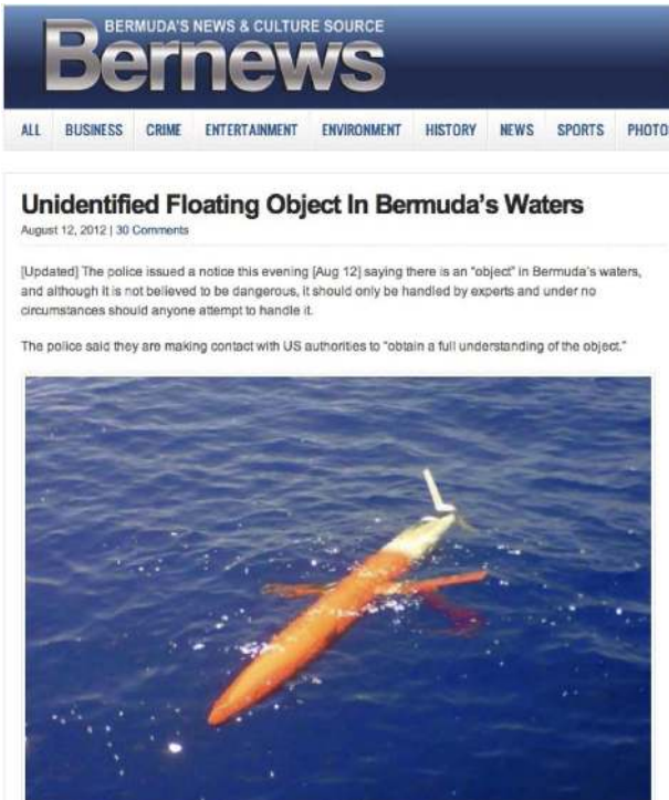
Fig. 8. The glider picture published in a Bermuda local news, under the title, “Unidentified Floating Object”. The spray glider was lost during a test near Bermuda. A reason of its malfunctioning is still unclear. A person on a yacht accidentally found the glider and took a picture 10 hour after our team officially determined its lost. Glider operation requires close communications among teammates and extensive preparations
