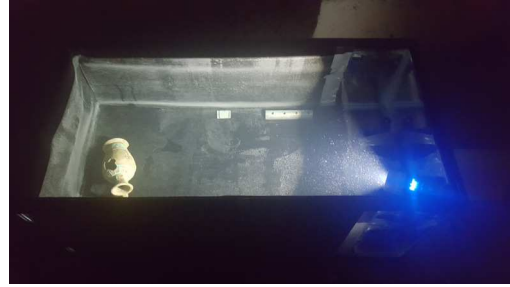
Figure 6. Experimental setup with in-lab water tank in controlled lighting environment with a single direct lighting source. The light field camera is placed flush to the tank wall for imaging an artificial scene a distance of approximately 1m from the camera. Milk is added to the pure water tank to simulate effects of backscattering present in field experiments.
