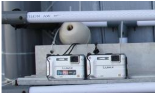
Figure 5: Low Cost Multi-View Camera Installation
