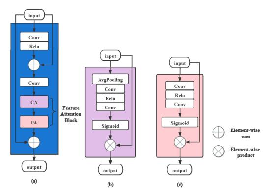
Figure 6. (a) Basic Attention Block (BAB); (b) Channel Attention (CA); and (c) Pixel Attention (PA).
