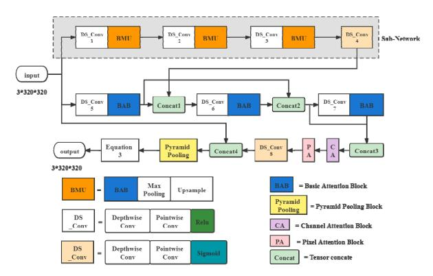
Figure 5. The end-to-end defogging network structure.
