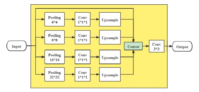
Figure 7. Pyramid pooling block.
