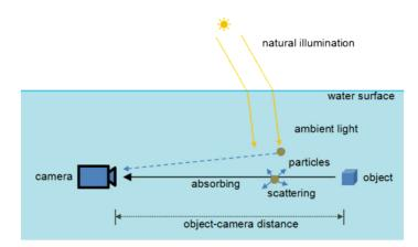
Figure 1. Underwater imaging model.
