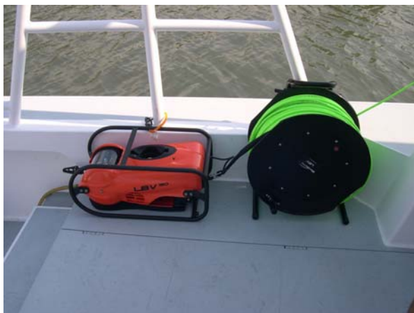
Fig 2: The Seabotix LBV Remotely Operated Vehicle
