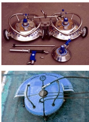
Figure 6. Cavitation system,CAVI-JET Pistols and Robot [25]
