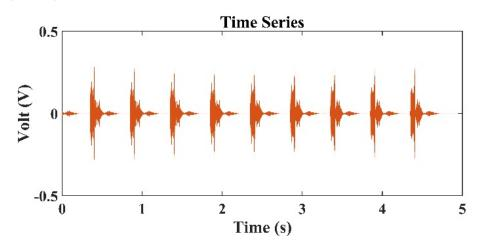
**Figure 3.** Typical time series of signals received by the second hydrophone ( $h_2 = 1.5 \text{ m}$ ) in the TRM, which is 80 m from the sound source of 3 kHz.
