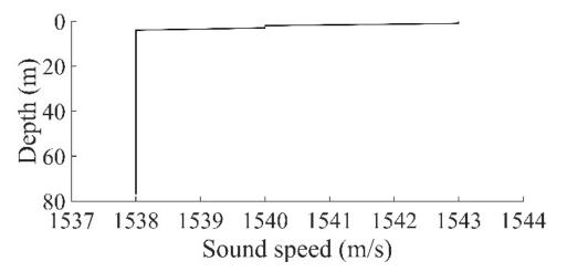
Figure 6. Sound velocity profile at the test location in the offshore region off Small Liuqiu Island.
