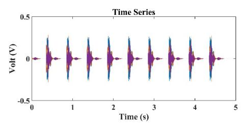
**Figure 4.** Typical time series of signals received by all hydrophones in the TRM, which is 80 m from the sound source.
