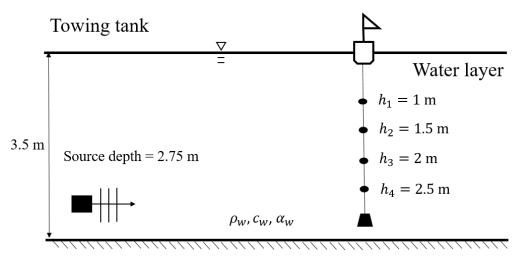
**Figure 2.** Layout of laboratory tests in the towing tank. The interval between two adjacent hydrophones is 0.5 m, the interval between the topmost hydrophone and the water surface is 1 m, and the interval between the bottommost hydrophone and the tank bottom is 1 m.
