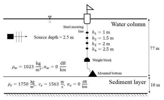
**Figure 7.** Parameters and geometry of the TRM experiments conducted in the offshore region off Small Liuqiu Island.
