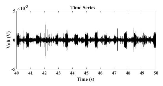
**Figure 11.** Time series of signals received by the third hydrophone in the TRM, which was 1.6 km from the sound source with a frequency of 3 kHz.
