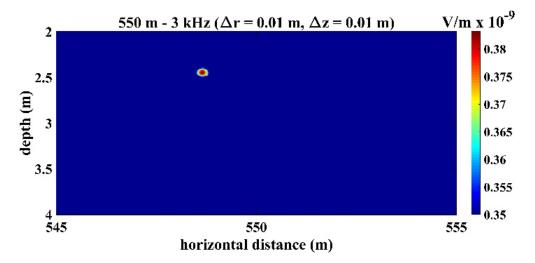
**Figure 10.** Sound pressure at the retrofocused location in the domain near the sound source, which locates at  $r_o = 550$  m and  $z_o = 2.5$  m. The result indicates that the estimated source location was  $r_{oe} = 548.6$  m and  $z_{oe} = 2.45$  m.
