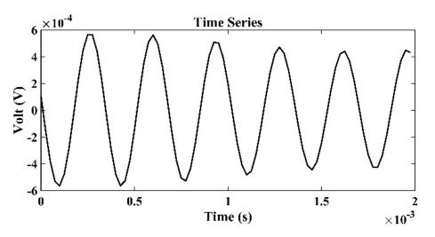
**Figure 9.** Time series of sound signals within  $2 \times 10^{-3}$  s that were received by the third hydrophone in the TRM, which was 550 m from the sound source with a frequency of 3 kHz.
