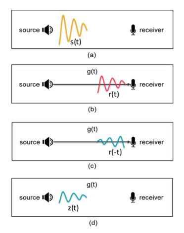
**Figure 1.** A time-reversal mirror (TRM) in the time domain. (a) Sound source signal s(t), (b) received sound signal r(t), (c) time-reversed signal of r(t), and (d) signal received at the location of the probe source.
