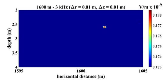
**Figure 12.** Sound pressure at the retrofocused location in the domain near the sound source, which locates at  $r_o = 1600$  m and  $z_o = 2.5$  m. The result indicates that the estimated source location was  $r_{oe} = 1601.9$  m and  $z_{oe} = 2.60$  m.
