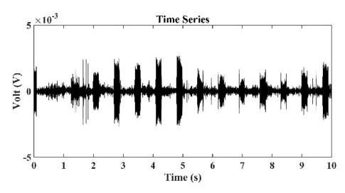
**Figure 8.** Time series of signals received by the third hydrophone in the TRM, which was 550 m from the sound source with a frequency of 3 kHz.
