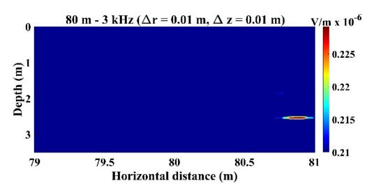
**Figure 5.** Sound pressure at the retrofocused location in the domain near the sound source, which locates at  $r_o = 80$  m and  $z_o = 2.75$  m. The result indicates that the estimated source location was  $r_{oe} = 80.89$  m and  $z_{oe} = 2.54$  m.
