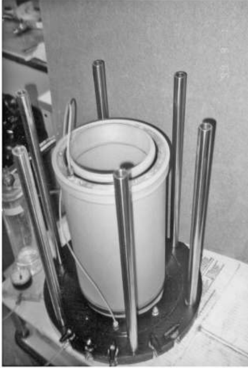
Fig. 2. Set-up of a hollow cylindrical sample
