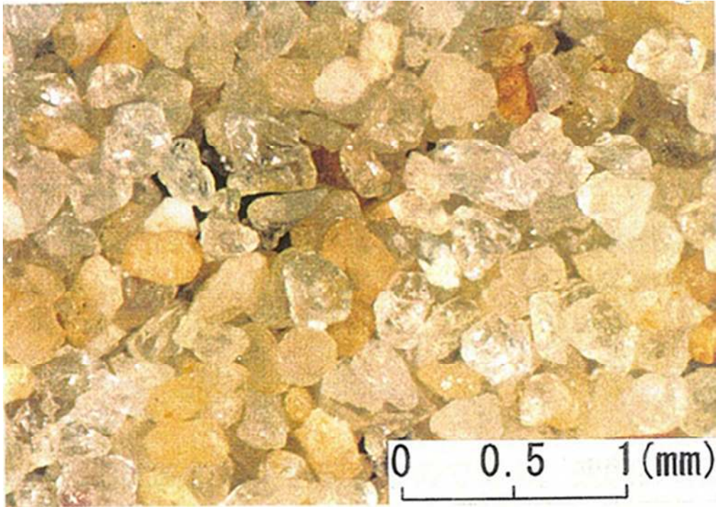
Fig. 2 Optical microscope image of Aio sand
