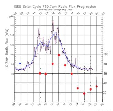
Fig. 14 Occurrence rate of VLF bursty-patches at frequencies above 6 kHz at KAN in 2012–2021 and the solar cycle activity (2008–2021) shown via F10.7 cm Radio Flux Progression
