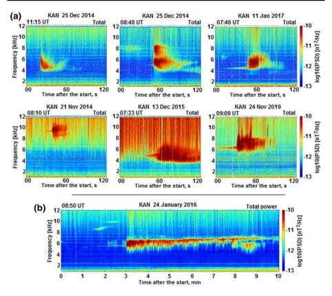
**Fig. 11** (a) Six examples of 2-min spectrograms of different VLF triggered-like patches observed at KAN; (b) a 10-min spectrogram shows quite sharp upper cutoff of the event near 7 kHz
