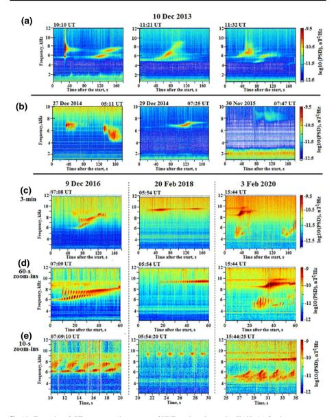
**Fig. 12** Examples of different spectral structures of VLF patches observed at KAN. (a) 3-min spectrograms of the VLF patches with a sharp low frequency cutoff on December 10, 2013. (b) Typical spectral shapes of the VLF patches. (c)– (e). Very complicated spectra of the VLF patches on three different days; (c) 3-min spectra (d) 1-min spectra detailing 3-min events; (e) Same in 10-s scales. Adopted from Manninen et al. (2021)
