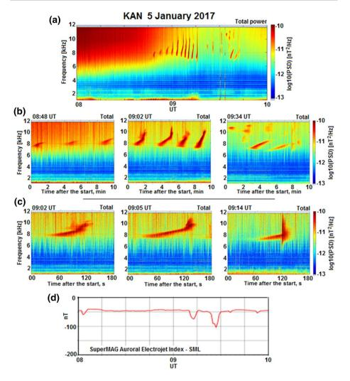
**Fig. 7** An example of spectral evolution of the dash-like VLF bursts from ~08:40 to ~09:50 UT at KAN on January 5, 2017, between 08 and 10 UT: (**a**) 2-h total power at 08–10 UT; (**b**) and (**c**) 10-min and 3-min spectrograms selected during the studied event (description in the text); (**d**) 2-h geomagnetic activity representing the SuperMAG auroral electrojet *SML*-index
