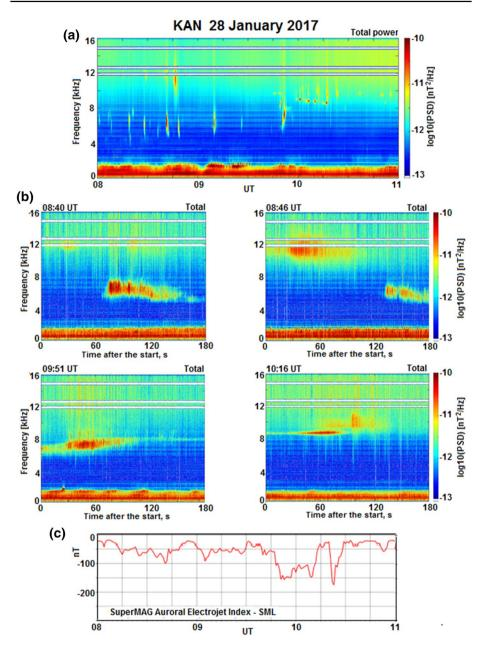
Fig. 8 (a) A 3-h total power spectrogram on January 28, 2017. Triggered bursty-patches below 8 kHz were observed mainly before local noon (~10 UT) and "dash-like" emissions above 8 kHz were observed mostly after noon; (b) 3-min spectrograms before and after the local noon; (c) The geomagnetic activity representing the SuperMAG auroral electrojet *SML*-index
