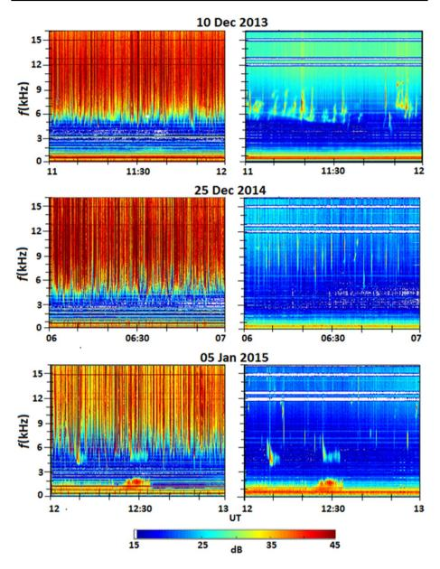
**Fig. 1** Examples of 1-h dynamic spectrograms (0–16 kHz) of non-filtered (left panels) and filtered (right panels) VLF data at KAN during three different days. White horizontal lines above 11 kHz in the right panels are the removed radio navigation transmitter signals. Taken from Manninen et al (2016)
