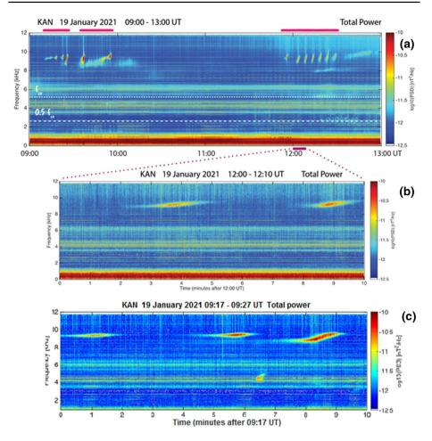
**Fig. 5** Another example of the series of dash-like VLF bursts observed at KAN on January 19, 2021: (a) between 09:00 and 13:00 UT and (b) between 12:00 and 12:10 UT (in the end of the event). (c) VLF emission from 09:17 to 09:27 UT (in the beginning of the event) showing "S-shape" "dash-like" emissions. Figure is also reproduced from Martinez-Calderon et al. (2021) with the addition of panel (c) showing another time frame of the event
