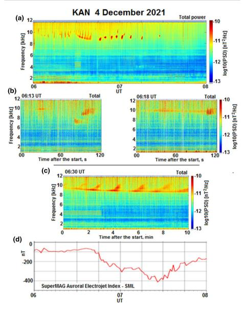
Fig. 9 (a) 2-h total power spectrogram at 06-08 UT on December 4, 2021; (b) 2-min spectrograms in the beginning of the event; (c) a 10-min spectrogram in the middle of the event; (d) the substorm activity according to the SuperMAG auroral electrojet *SML*-index
