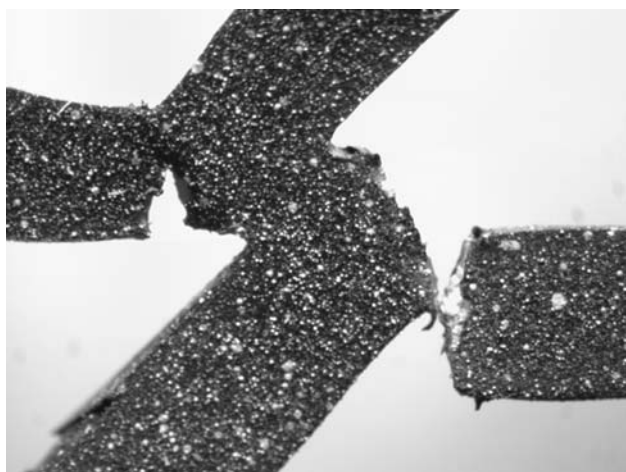
Fig. 15 Shear test coupon SC3a (GMT#90): failure in bending rather than in shear. The field of view of the entire image is 7.3 mm \times 5.5 mm
